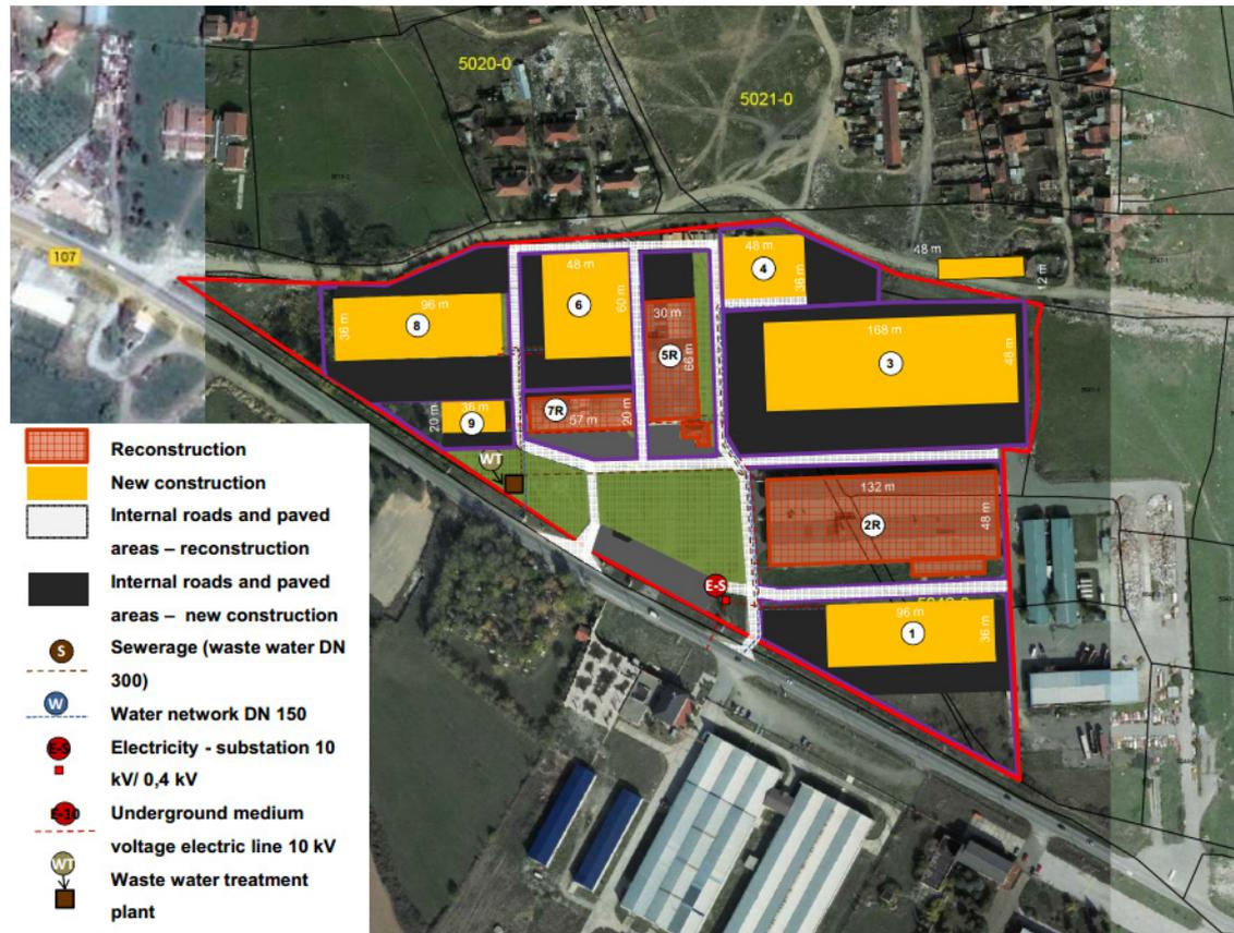
Figure 53 - Overview of future facilities to be located at Virxhinia site
